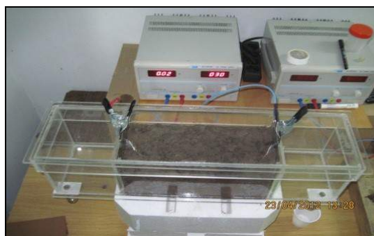
Fig. 1 - Experimental installation of electro-flushing (top view)
